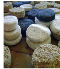
Biomass sawdust briquette
